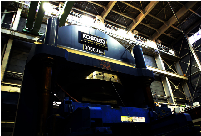
Figure 6. The 30,000-ton hydraulic press utilized at NIMS (Japan) for the High-Pressure High-Temperature (HPHT) synthesis of benchmark hBN crystals (Image adapted from NIMS MANA e-Bulletin) [5].
